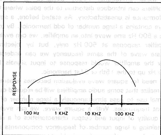
Fig. 13. Response curve of amplifier with poor low and high ends
