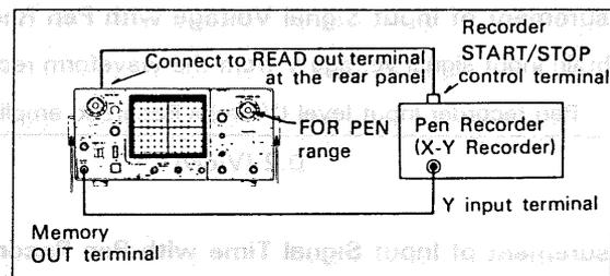
Fig. 5. Data recording with pen recorder
