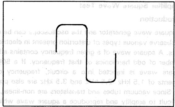
Fig. 12. Square wave response with high frequency loss
