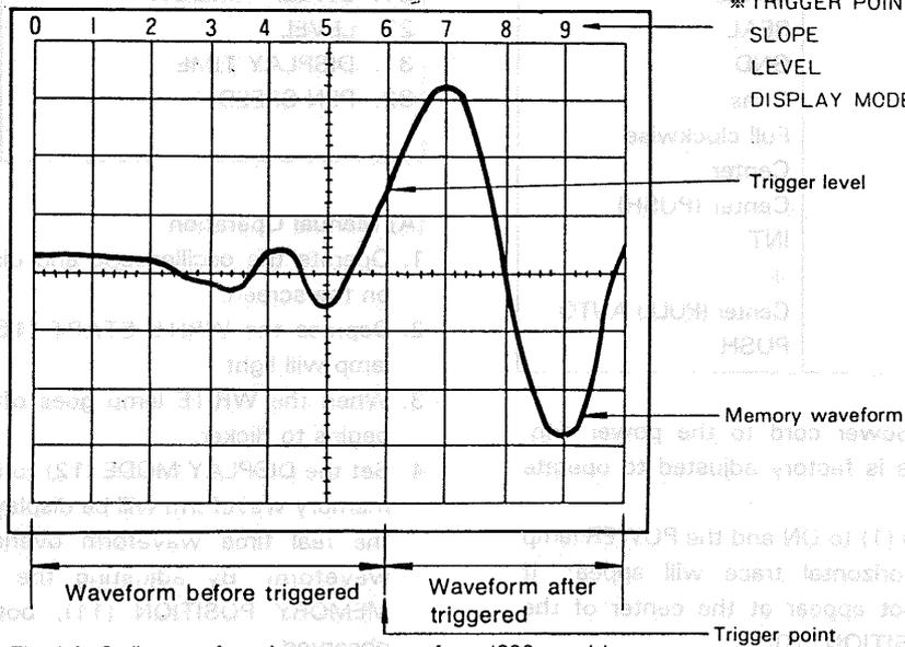
The left 6 div waveform is memory waveform (600 words) before triggered. The right 4 div waveform is a memory waveform (400 words) after triggered.
