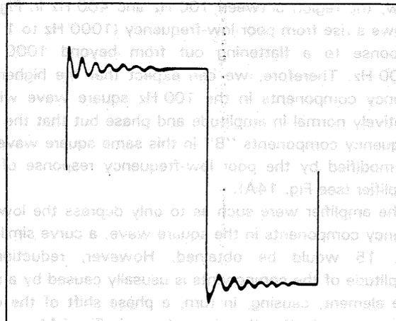
Fig. 21. Effect of high-frequency boost and good damping
